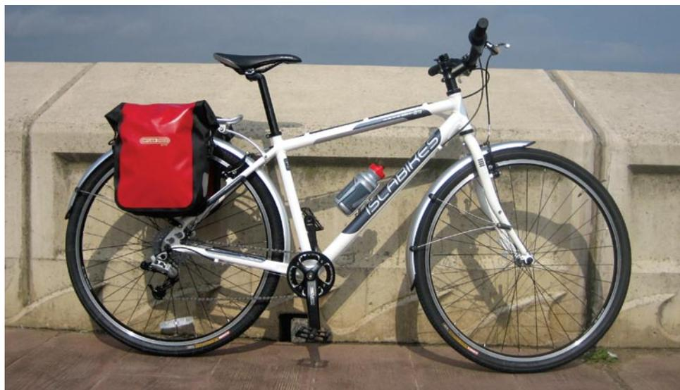
strengthen it here. The fork is rigid chrome-moly – a better and lighter option for any usage than a sub-standard suspension fork. A larger than normal offset (50mm) keeps the steering sharp and the front wheel further from your feet.
