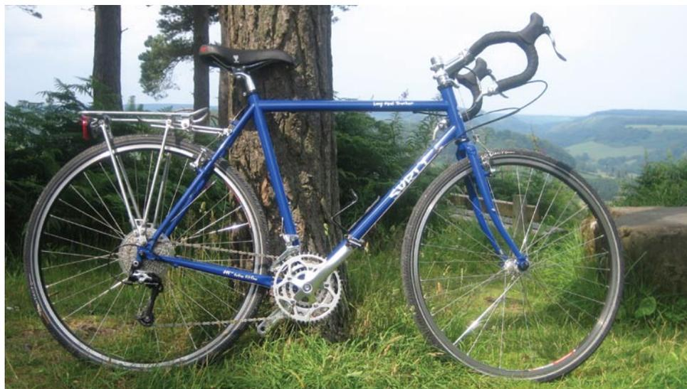
rather have 170mm, for while the LHT's low bottom bracket makes it easy to get a foot down, it can also result in pedal strikes on rougher tracks. And the LHT is a robust tourer that will readily tackle such terrain. A chain-stay transfer reads: Fatties Fit Fine. Tyres, that is! There's just clearance for 50mm, even with mudguards.
