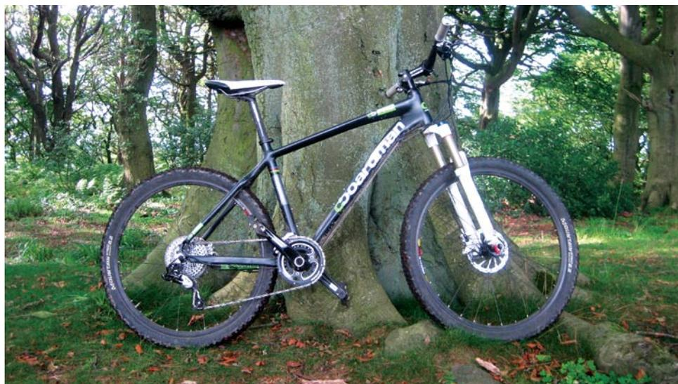
you can set the positive and negative air springs precisely to your weight and preference. Its tapered steerer means it has a bigger (1.5in) lower headset race, which should reduce steering flex and lengthen bearing life.
