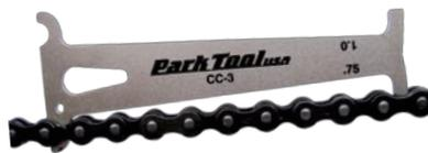
direction of the chain changes nothing much, but flipping laterally, so the side nearest the spokes is now away from them, may even up the effects of out-of-line running, which can sometimes wear one end of the pins more than the other. Topology rules that you can flip a chain simultaneously in any two of the three possible senses (inside-
