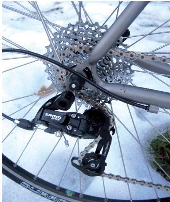
(Clockwise from above) Sram's Apex 11-32T cassette is a perfect match for a compact double chainset, widening the range significantly. The Audax's frame and fork have been designed to utilise all the drop available from 57mm brakes. That's a size 8 shoe and it's a 54cm frame.
