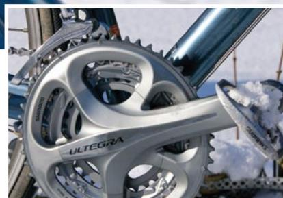
is a composite of alloy and carbon-fibre-polymer with a hollow core and concealed nuts that gives an even more streamlined appearance to the chainset now.
