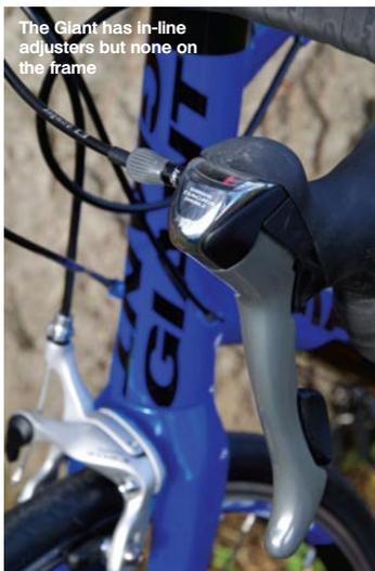
The Giant has in-line adjusters but none on the frame
