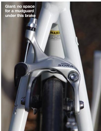
Giant: no space for a mudguard under this brake
