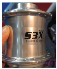
Sturmey-Archer had resurrected two old hubs: a three-speed fixed hub, the S3X (1st 0.625, 2nd 0.75, 3rd 1:1); and a new take on the old Sachs Duomatic, the cable-less S2C Kick Shift (1st 1:1, 2nd 1.38). www.sturmeyarcher.com, www.moultonbicycles.co.uk
