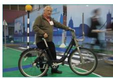
Transport for London's new cycle hire bikes were available to try on the test track. They've got Nexus 3-speed hub gears, concealed cables, dynamo lights, and roller brakes. There's a partial chainguard (a shame not to have a full guard) and a skirt
