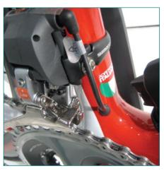
Shimano's electronic Dura Ace, Di2, was first shown last year. This year it was fitted to a few show bikes, notably this De Rosa. The electric cables that Di2 uses are neatly routed internally, though the Li-ion battery is still external. How long will the latter last per charge? 'One Grand Tour', say Shimano. www.shimano.com
