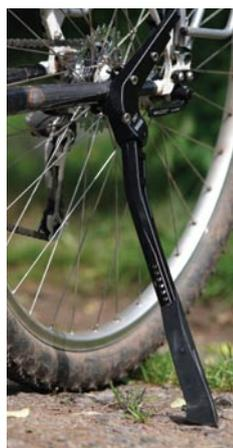
Kickstands can be surprisingly useful when touring. At 473g, the Multi Zoom will add heft to your bike, but it is tough enough to support one laden with four panniers. It fits a range of frame sizes, thanks to adjustability in the leg, and is braced across the seat and chainstays; the chainstay clamp is also adjustable depending on tubing size or disc brake tabs. In use, the Multi Zoom works very well and saves scuffing your panniers on the ground
