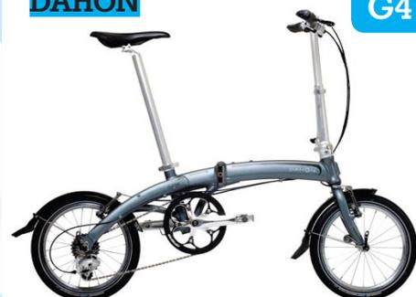
Dahon's Curve SL is a sub-10kg hub-g geared commuter folder that rides very well thanks to its Schwalbe Big Apple tyres, which eat bumps that can upset small-wheeled bikes and which provide an excellent level of shock absorbency. The fold is obvious and makes the bike quite compact so it's a good option for bike-rail users, who need hassle-free boarding.
