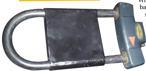
After reading the security article in the Feb-Mar issue of Cycle, I asked a local smithy to make for me a lightweight steel box to fill the inside of my D-lock to prevent access with a 'stubby' bottle jack. It is made from thin-gauge steel, MIG-welded, and slips on between bike and locking post as shown.
