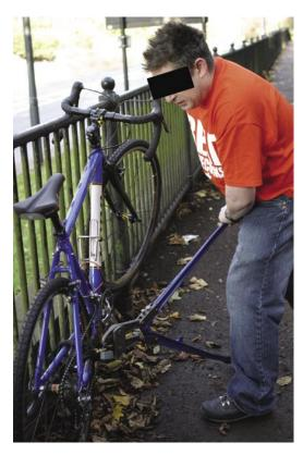
Snip! With 36-inch bolt croppers, the than 2 seconds. The one opposite lasted 10.6 seconds to mere cable cutters
