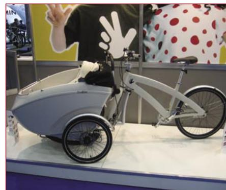
The Danish Triobike is a child/load-carrier trike that separates a bit like a Rollfiets wheelchair tandem to give a bike (spare front wheel carried underneath) and a push-along buggy. The buggy can fit a seat designed for babies as young as 3 weeks. It costs around £2200. More at [www.triobike.com](http://www.triobike.com)
