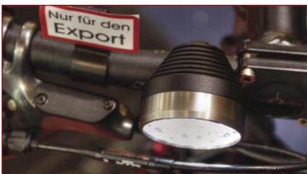
Major improvements in the efficiency of white LEDs were made during 2007. The latest emitters can now yield up to 90 lumens of light per electrical watt. That's three times the efficiency of the best halogen bulbs and 50% better than a HID lamp. Since LEDs also last a great deal longer than either of the above, and unlike them can be efficiently dimmed for further economy or to avoid causing dazzle, the
