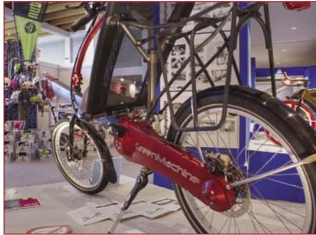
of their clean, green recumbent pedalling machine. A specially modified Rohloff hub provides an intermediate gearbox, coaxial with the rear suspension pivot and transferring chain drive from the right side to the left. A two-legged fork rather spoils the asymmetry, but a monoblade is in development. See [www.flevobike.nl](http://www.flevobike.nl)
