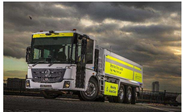
"Direct vision" lorry cabs, in which drivers can see what is around them as easily as a bus driver can, with the driver seated down low and surrounded by as much window as possible.
