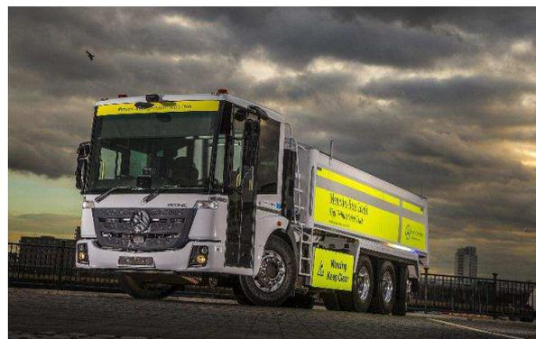
"Direct vision" lorry cabs, in which drivers can see what is around them as easily as a bus driver can, with the driver seated down low and surrounded by as much window as possible.
