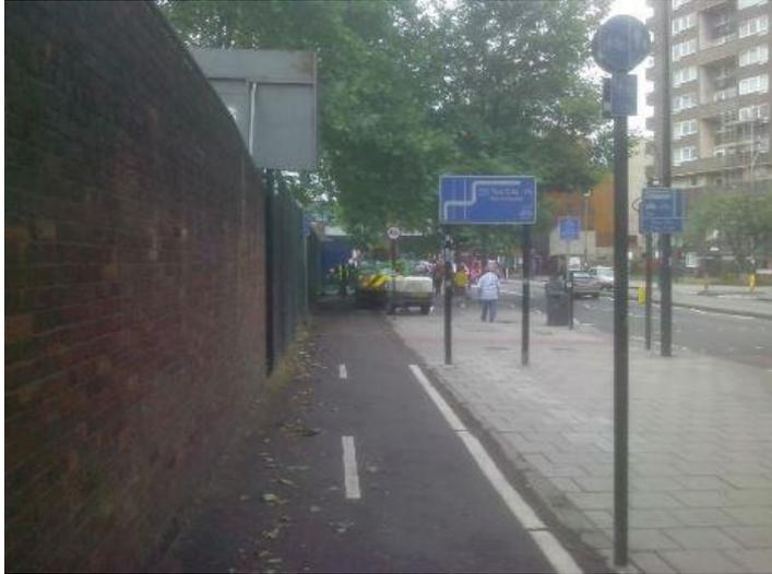
Photo 3: the same scene looking westbound. The nearest sign indicates that the area up to and beyond the pelican crossing (as far as the "no cycling" sign in the background) is a segregated track. This not only contradicts the sign in the foreground of photo 1, but also provides no indication of where cyclists may legally access the pelican crossing point, despite the direction signing urging them to do so.
