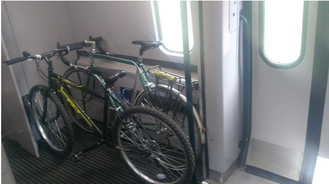
The Class 158 trains, operated by South Western Rail, Scotrail and others, have cycle spaces between the doors and the end of the carriage. This allows bikes to be unloaded and stored easily, and to be loaded again before alighting. The space can also be used for luggage storage, as well as allowing passengers to congregate around the door before alighting, thereby reducing dwell times at stations.
