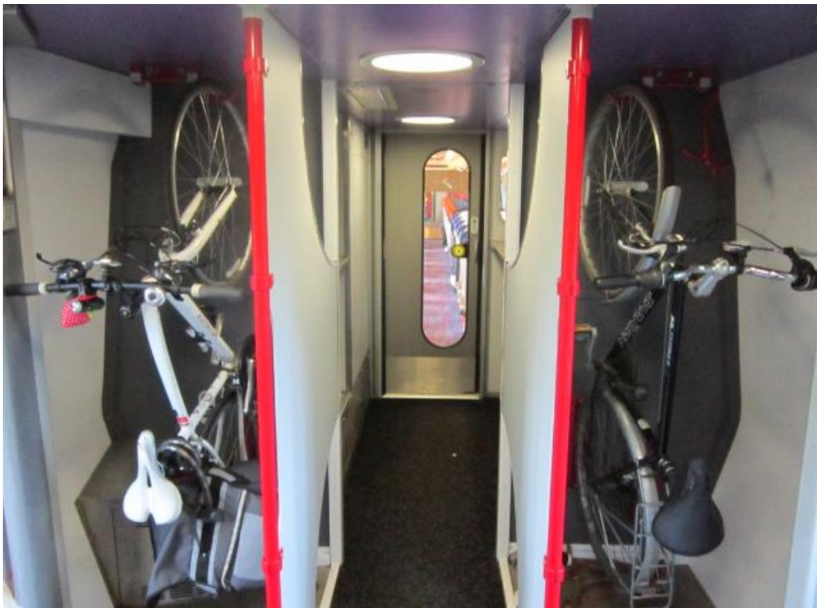
The Cross-Country 'Voyager' trains supposedly have space for 4 bicycles in two narrow compartments on either side of the corridor, adjacent to a door. However it is very difficult to manoeuvre a bike onto the hanging hooks in such a confined space when other passengers are trying to board or alight (all the more so if you also have to load or unload the bicycle), and impossible to fit in two bikes in each compartment unless they both have very narrow handlebars.
