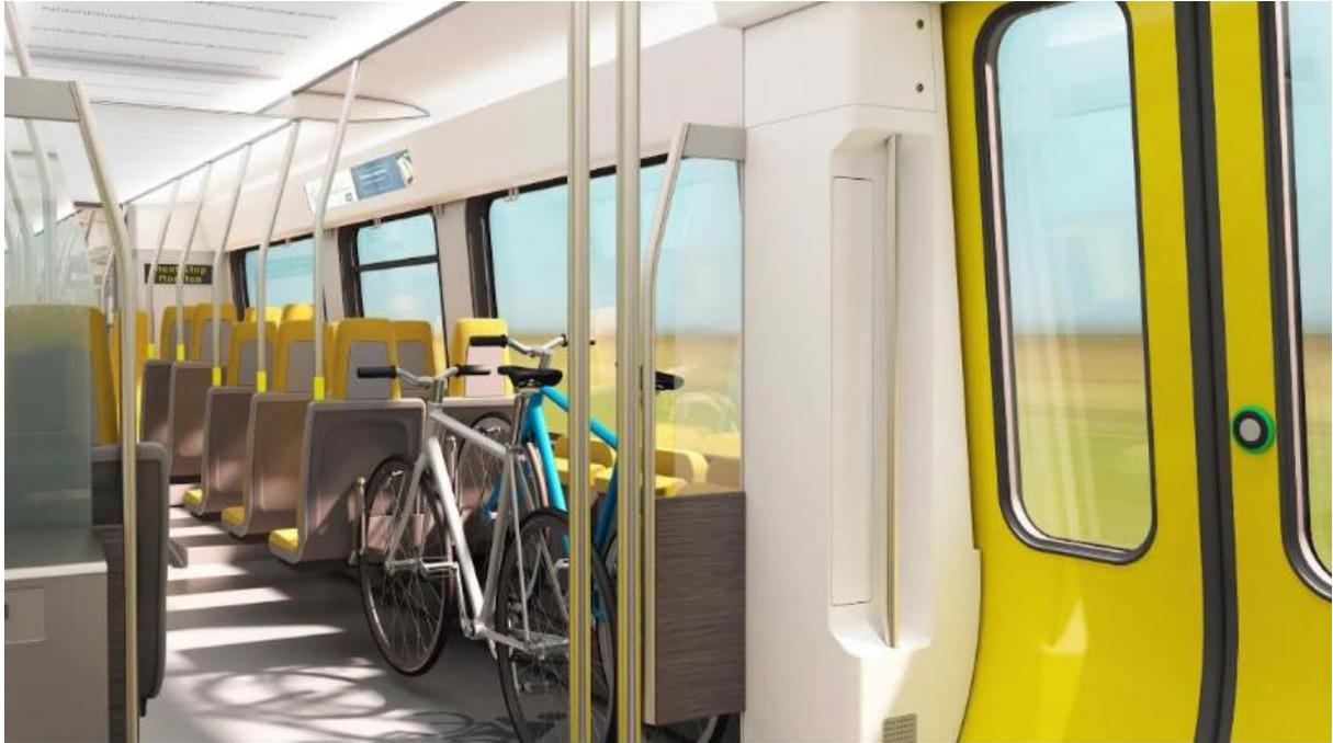
Merseyrail's new Stadler trains allow up to 3 bicycles to be stored in a space adjacent to the central double-doors. When not in use, the space can be used flexibly e.g. for storing buggies and other luggage, or as standing room at peak hours. Tip-up seats are also provided. A similar arrangement was devised by South West Trains (now South Western rail) in conjunction with Cycling UK and the London Cycling Campaign for the upgrade of its Class 455 trains (below).
