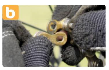
The link can then be joined by placing each rivet through the keyhole in the opposite plate and pulling the chain tight so the rivets secure themselves in the keyhole slots (c).
