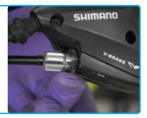
Wind the adjuster in or out as appropriate to find the correct lever position. Winding it out 'tightens' the brakes (moves the brake lever further away from the handlebars), winding the adjuster in, reduces the reach of the lever (for smaller hands).
