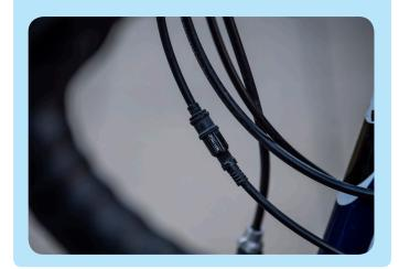
Barrel adjusters may be on the rear derailleur and/or the rear/right hand gear shifter (flat bar bike). There may be one on the right hand side of the frame or an in-line adjuster on the rear gear cable outer for road bikes.
