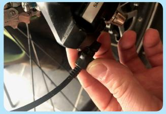
Rear/Right Hand Shifter Barrel Adjuster
