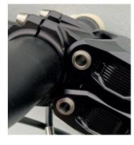
the stem does not 'top out' over repeated bumps. Instead, the handlebar simply floats around some intermediate point, with upward movement only seen when pulling up on a climb.
