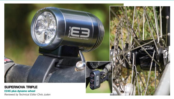
The Supernova E3 Triple is a dynamo headlamp from Germany intended for mountain biking. The factors that made dynamo lighting a non-starter off-road have been answered one-by-one by new technology.
