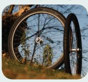
tours. The wheels themselves are built to Spa Cycle's typically high standards, laced with double-butted spokes all round, except on the rear driveside which uses Sapim Strongs for extra strength. The 36-hole rims also contribute to a tough, laterally stiff wheelset.
