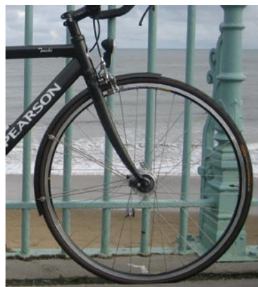
Carbon forks with eyelets and clearance for a mudguard are available
